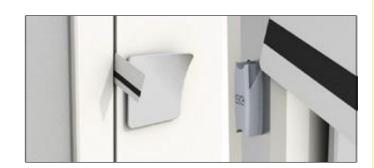
Insert a plastic card in the crack of the door at the lock's height, using it to feel for the top edge of the latch. Next, slide the bottom of the card into the recess on the side of the latch. Now pull down vertically up to stop on the door edge. The latch is now pushed in and the door can be opened. Only remove the card from the recess once you have opened it.
