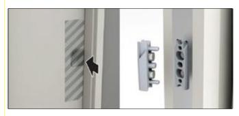
In the event of an emergency, if you cannot remove the door handle on the inside of the hinge, prize opens the door, applying serious force around the handle area. With 1 KN of force, the safety clip on the latch will yield and the door will open.
