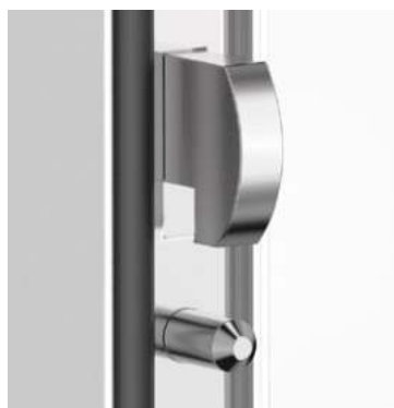
02 Swivel-type steel hook bolts protected against drill and saw attack by an auxiliary bolt.
